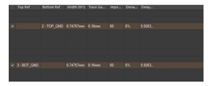
Here, you can see Top Ref is blank for the above row since that layer is implied to be 'Top Layer' from the stackup. Similarly, for the bottom row, the Bot Ref is implied to be 'Bottom Layer' from the stackup and thus is left blank.
