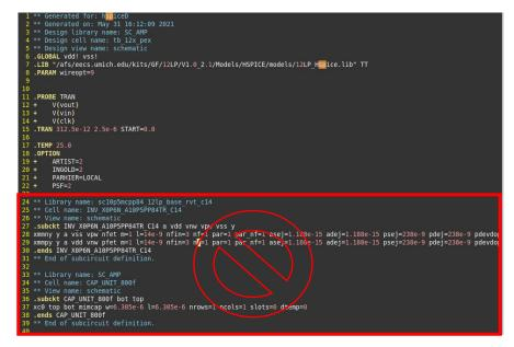
b. Remove .include and add finesim options (also add .include for your design\_name.pex.netlist)
