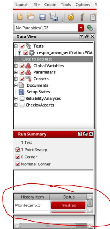
11. Finally, you must manually click plot all button (in the results tab), denoted as a line graph. For scalar data, it will plot the data as a histogram. You can also view the data in the results table by clicking the pull-down menu where it is default yield and select detail, to show the data point history of the analysis.
