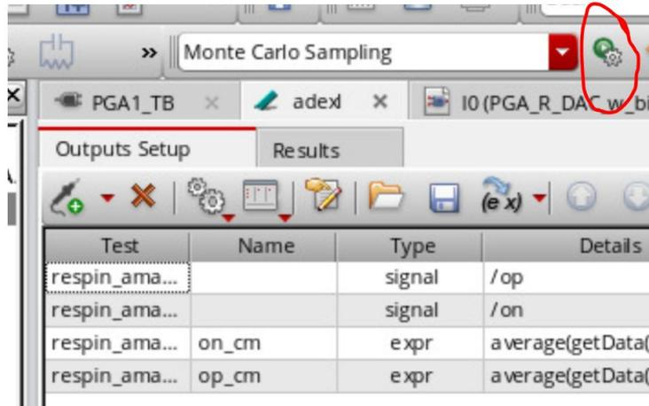
9. A popup should appear. Enter the number of points (how many different times monte carlo will simulate/ how many different variations). Make sure save mismatch data is check marked. Make sure save data to allow family plots is check marked. Enter a seed number (a value used for pseudo-random operation). Then click OK.
